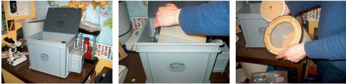
3. Now you have removed the drum you can open it to insert your leaf material. The lid of the drum is magnetically attached so you may need to firmly pull it off. Make sure that your plant material consists of only small leaves and flowers and not any stalks which may damage the screen of the drum. Close the lid of the drum and then put the drum back in the Pollinator.
